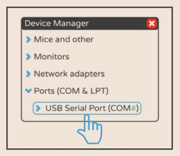
2 Navigate to the Device Manager on the PC and find the number of the COM port for the connection.
