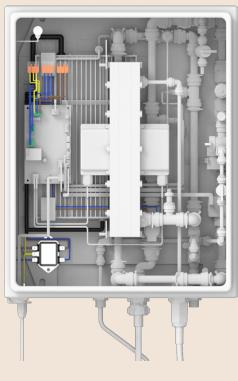
Mains power supply inputs through the IEC port, transfers through the line filter then runs to the PCB.
