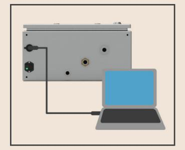
Connect a USB-B cable to the port on the underside of the SC-100. Connect the USB-A end of the cable to the PC.
