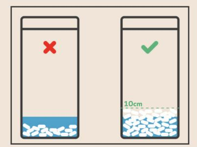
2 If the salt level is below the water level, more salt tablets should be added to a depth of approximately 10cm.
