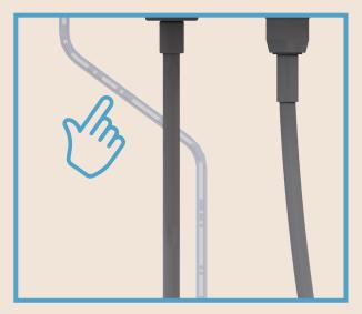
To solve this error, you should first follow the brine tank and softener SOP (page 25), which will allow you to check if there is enough brine in the tank itself and if the brine line is submerged in the brine solution. Once
