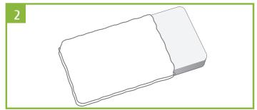
Place the Fripura unit into the unit bag and fold down the open end before placing into the metal case.
