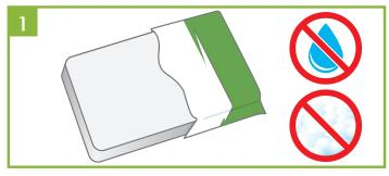
Once the packaging has been opened **do not** allow the unit to come into contact with steam or water.
