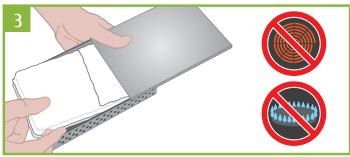
Load each new unit into the custom FriPura metal case. Do not use the FriPura unit without the metal casing. Do not place the loaded case directly onto electric elements or gas burner upstands.
