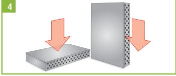
Close and place the loaded case into the fryer, prior to refilling with fresh oil. Either lay flat or stand on its narrowest width to ensure the casing holes are not covered.
