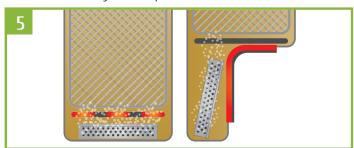
Ensure the unit case is fully covered by cooking oil during use and that the holes in the case do not become blocked *e.g. with food debris* During the first time of use the unit will bubble for a short time as the oil heats up. This is normal. The drawings above are indicative only. Fryers and placement of the FriPura filter and case will vary.
