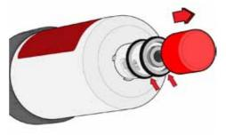
Insert new cartridge and turn until it locates. Install with a quarter-turn to the right until cartridge comes to a complete stop (Inlet water will automatically turn on). Close filter-door.
