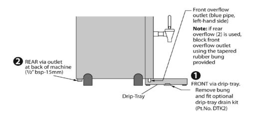
IMPORTANT: Whichever overflow connection is chosen, the diameter of the pipe used must be no less than 15mm.
