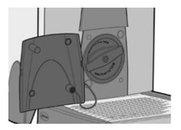
3. Grip Cartridge and rotate a quarter-turn to the left and pull forward. CAUTION: A small amount of water will drain from the head.
