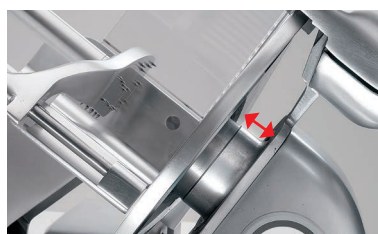
Increased gap between blade and machine body
