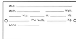
FIG. no. 4 - Rating plate - serial number
