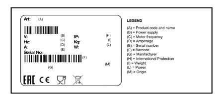
FIG. n°4 - Rating plate - serial number
