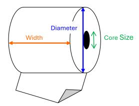
All measurements shown are Width followed by Diameter then the Core size (the hole in the middle) You can check the dimensions of the roll you require using the above diagram for guidance.
