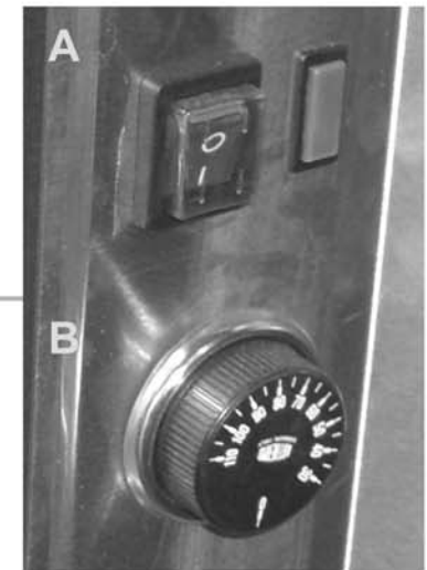
Mains Power (A) + Heat Control (B)
