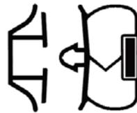
Door gaskets should be checked and cleaned regularly and replaced if damaged. To clean the gasket, wipe with warm soapy water and a soft cloth, ensuring it is completely dry before closing the door. **DO NOT** use a sharp knife to clean or scrape the gasket. Damaged gaskets do not seal correctly and can increase the amount of electricity consumed, seriously affecting the efficiency and performance of the cabinet.
